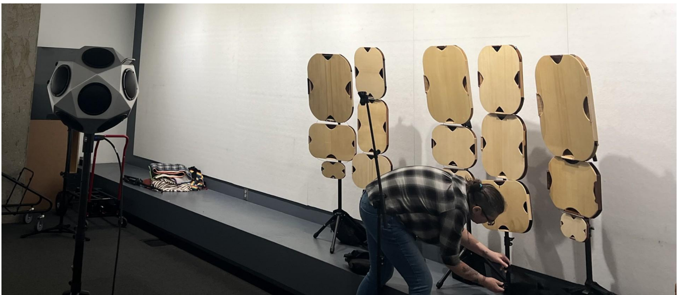
Rachel Ellison-Lee learned to use acoustic evidence as a design tool, developing resonant panels for a music-venue retrofit and validating their performance through physical measurements. Photo Credit: Rachel Ellison-Lee (top), Alaa Algargoosh (bottom)
